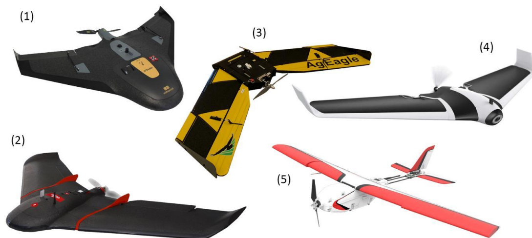
Slika 33. Dronovi nepokretnih krila: (1) UX5 Multispectral (Trimble); (2) eBee SQ (SenseFly); (3) Ag Eagle RX48 (AgEagle); (4) Disco-Pro AG (Parrot); (5) Lancaster 5 (PrecisionHawk) (Krevh, 2018).
