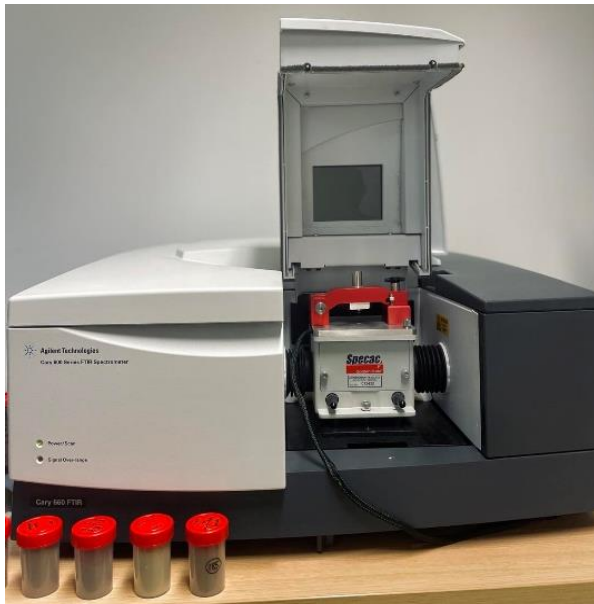
Figure 7. The FTIR-ATR spectrometer setup with the Agilent Technologies Cary 660 FTIR Spectrometer and single-reflection diamond ATR accessory *.
