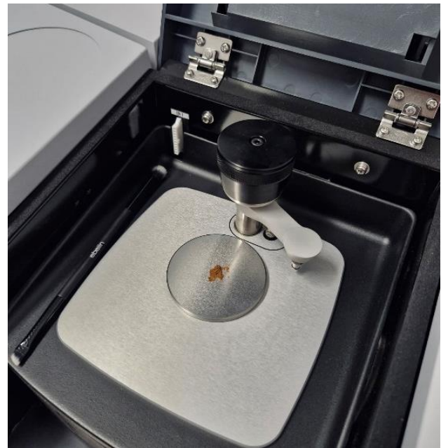
Figure 8. The FTIR-ATR spectrometer setup with the Shimadzu IRTracer 100 Spectrometer and single-reflection diamond ATR accessory **.
