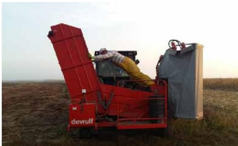
Figure 3. Machine for extraction Dewulf P3B (Source: Glogovšek, 2016)
