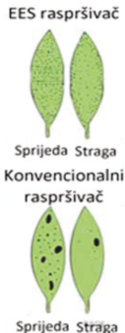
Figure 5. The principle of distribution of electrostatically charged particles on the leaf mass (Source: sprayers101.com )
