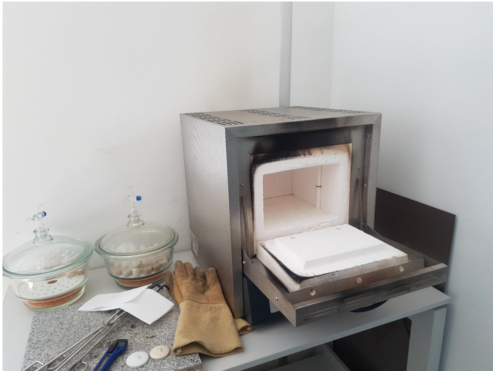
Slika 10. Mufolna peć marke Nabertherm Controller B170
