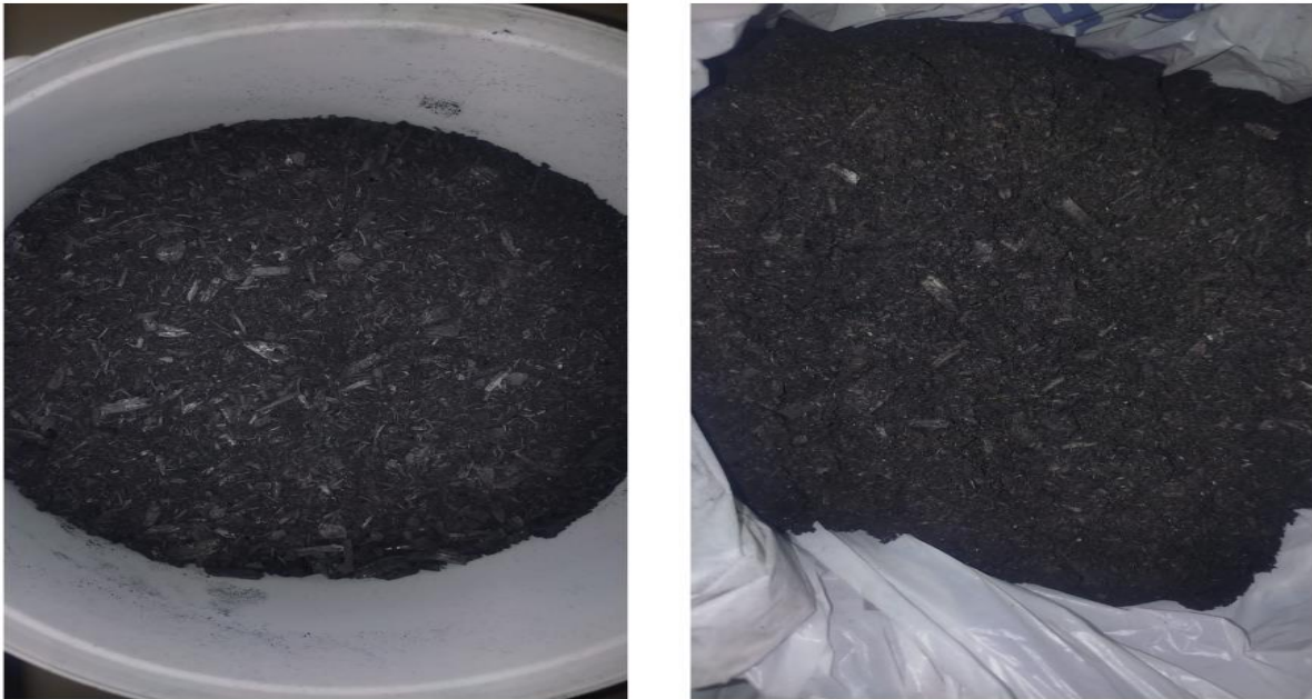
Figure 1. Presentation of wood chip-derived biochar (BC1, left) and horse manure-derived biochar (BC2, right)
