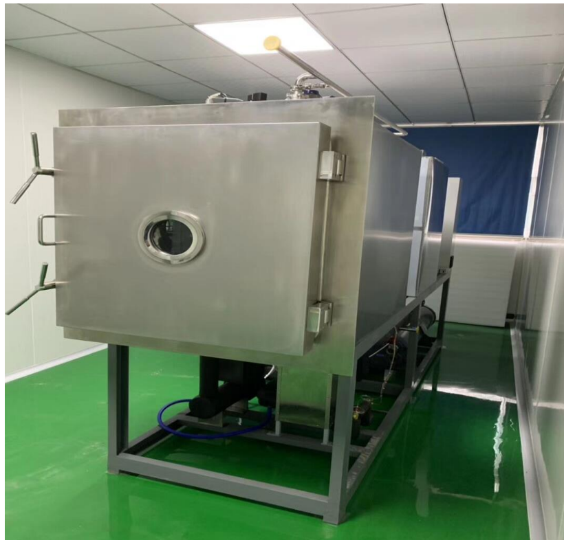
Slika 4. Liofilizator ( izvor: http://m.hr.cnscentz.com/news/new-use-of-flower-freeze-dryer-25066896.html )
