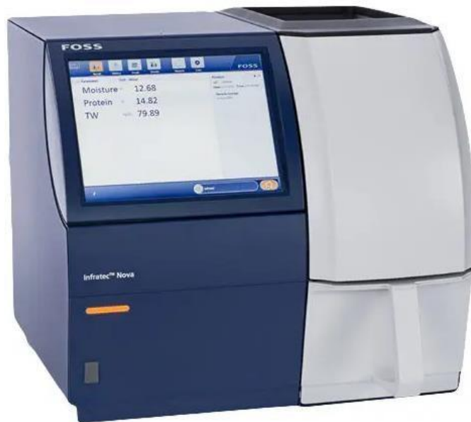
Slika 3.3.5. Infratec TM 1214 Grain Analyzer.
