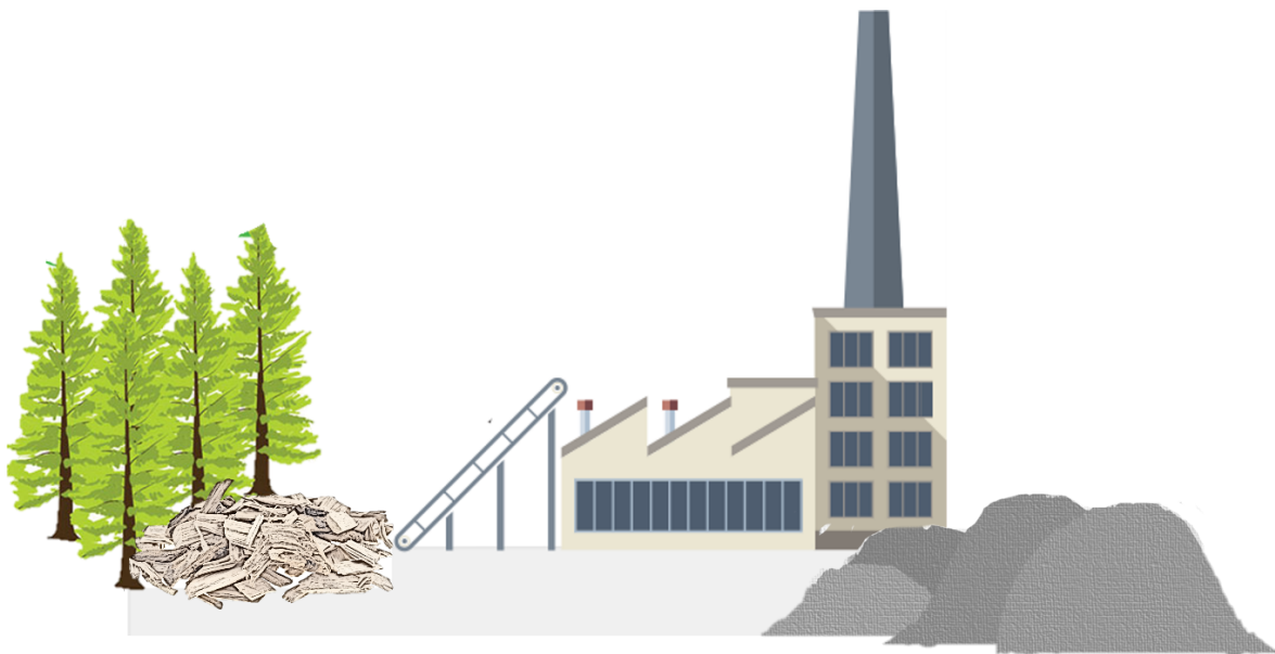
Figure 2.1.1.1. Biomass-fuelled cogeneration plant producing both electricity and heat, with bioash as a side product
