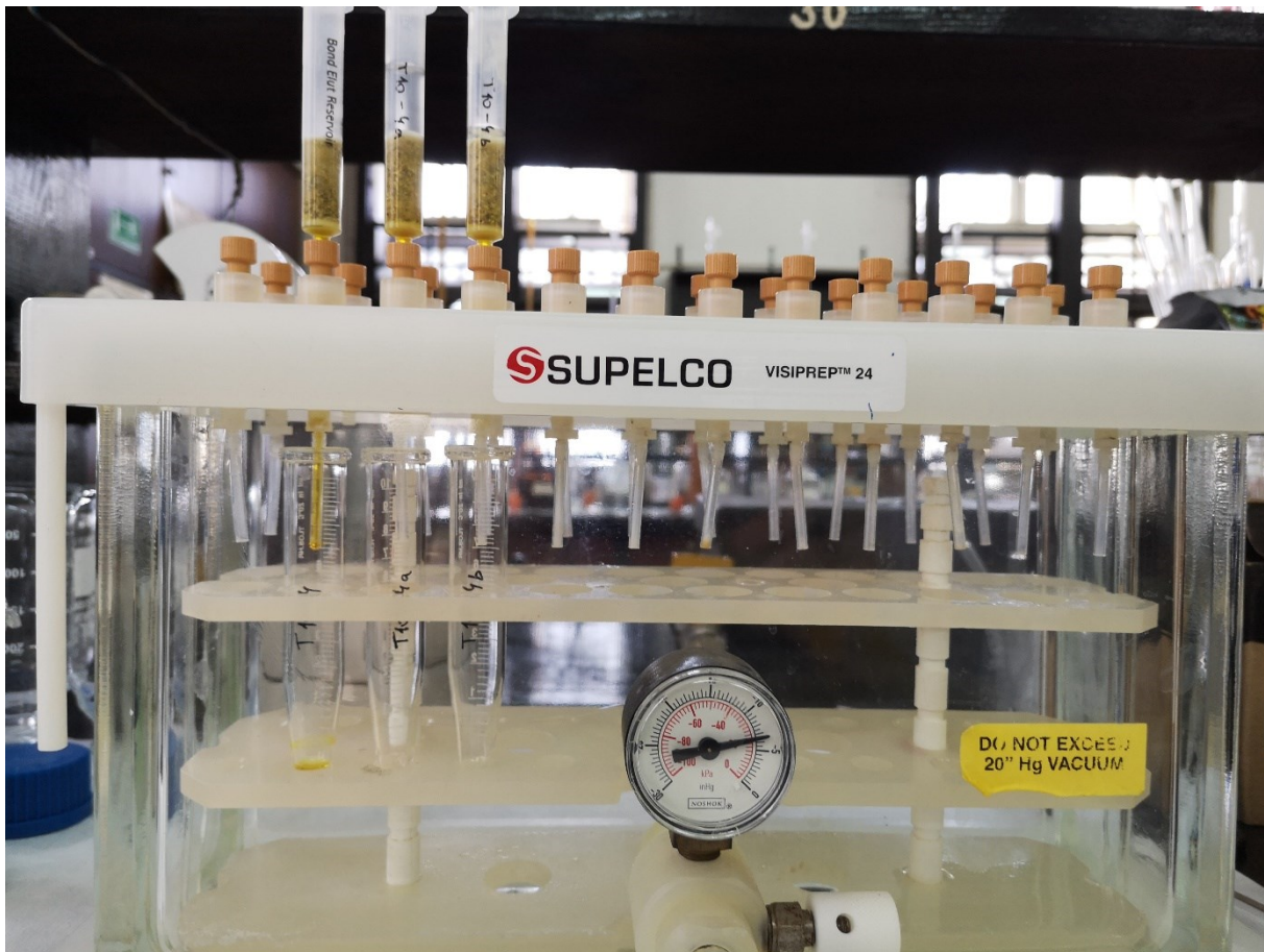
Figure 11. Extraction of pyrethrins using the SPE vacuum manifold.
