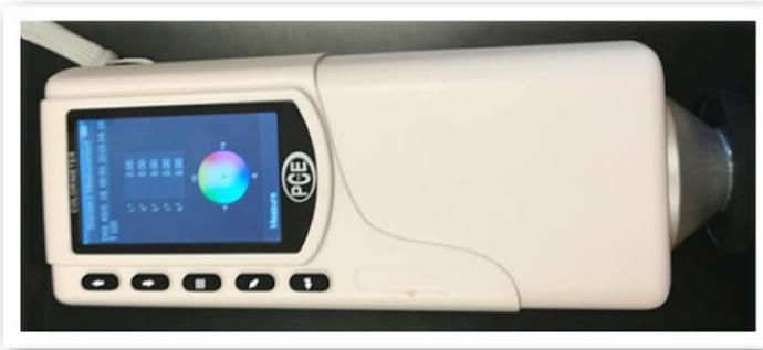
Slika 1. Kolorimetar (PCE-CSM2, PCE Instruments UK Ltd.)
