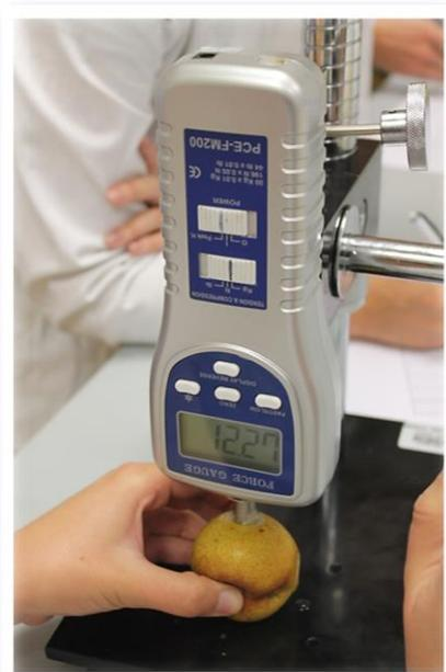
Slika 5. Digitalni stolni penetrometar (PCE-PT200, PCE Instruments, Southampton, UK)
