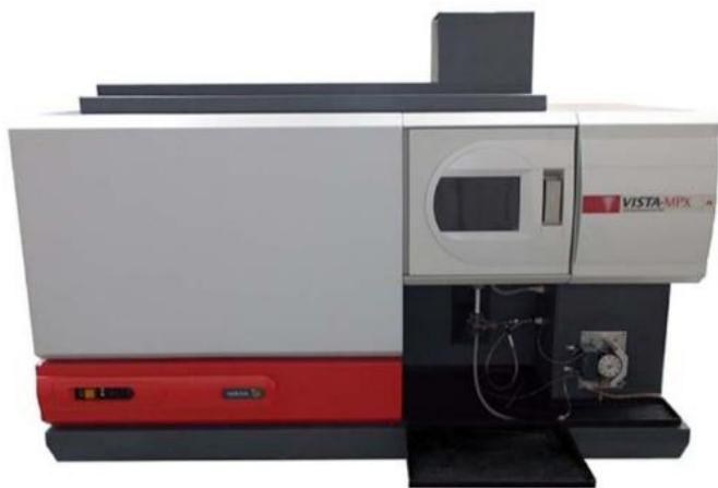
Slika 3.3.2.1. Spektrometar Vista MPX Simultaneous ICP-OES, Varian Inc.
