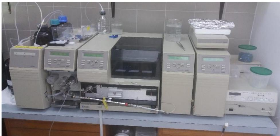
**Slika 13.** HPLC sustav SpectraSystem (Thermo Separation Products, Inc., SAD)
