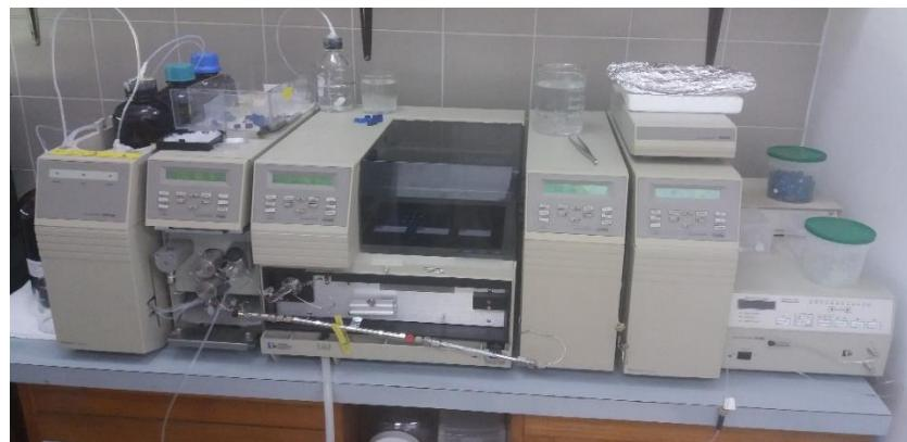
Slika 12. HPLC sustav SpectraSystem (Thermo Separation Products, Inc., SAD)
