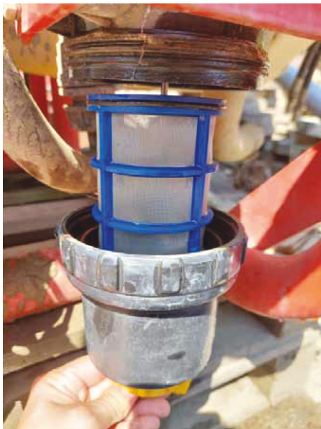
Slika 9. Filter prskalice Figure 9. Sprinkler filter
