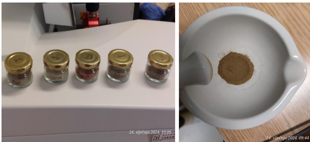
Figure 9. Preparation of soil samples prior to FTIR analysis: Five soil samples (Regosol acric, Dystric Stagnosol, Luvisol, Chernozem, Gleysol vertic (from left to right) and pulverization into fine homogenates using a mortar.
