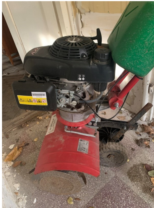
Figure 5.18 Rotary hoe (E. Takács)
