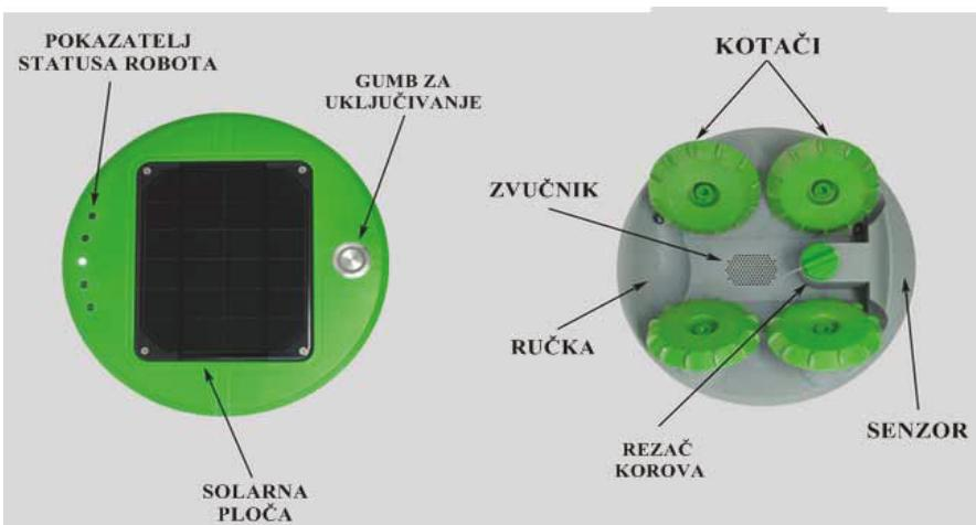
**Slika 13.** Dijelovi robota Tertill (Izvor: [www.robot-advance.com/EN/actualite-robot-gardener-tertill](http://www.robot-advance.com/EN/actualite-robot-gardener-tertill))
