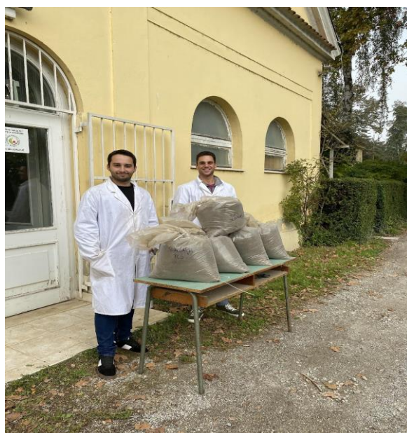
Figure 2. Contaminated soil after being sieved to < 2 mm and before being mixed into pots
