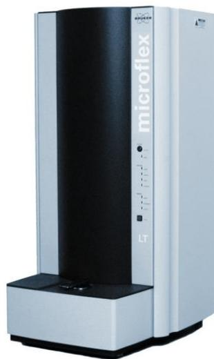
Slika 4.3.1. Prikaz MALDI-TOF spektrometra masa (microflex MALDI Biotyper Bruker)
