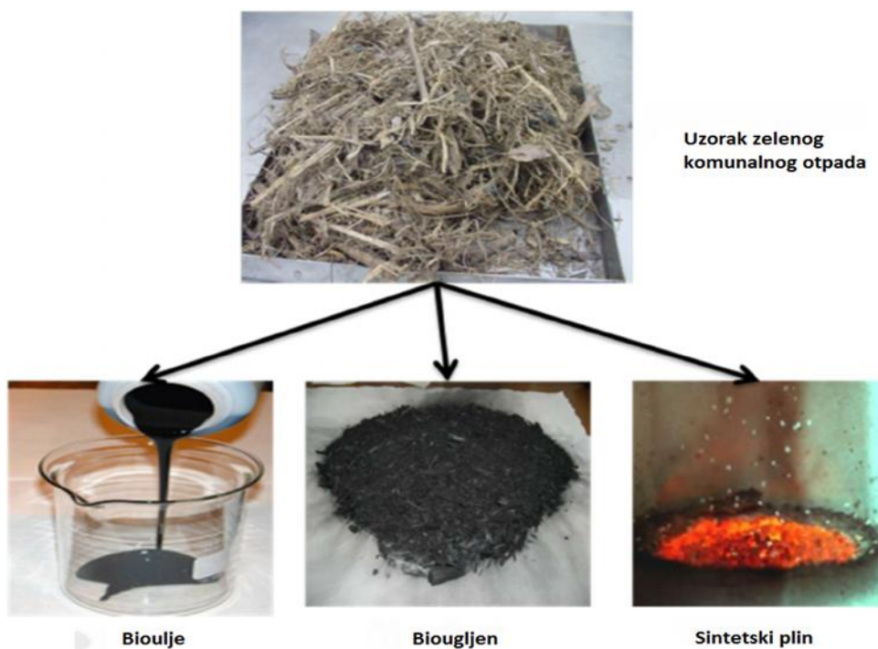
Slika 2.2.2.1. Produkti pirolize (Izvor: www.mdpi.com/journal/energies )
