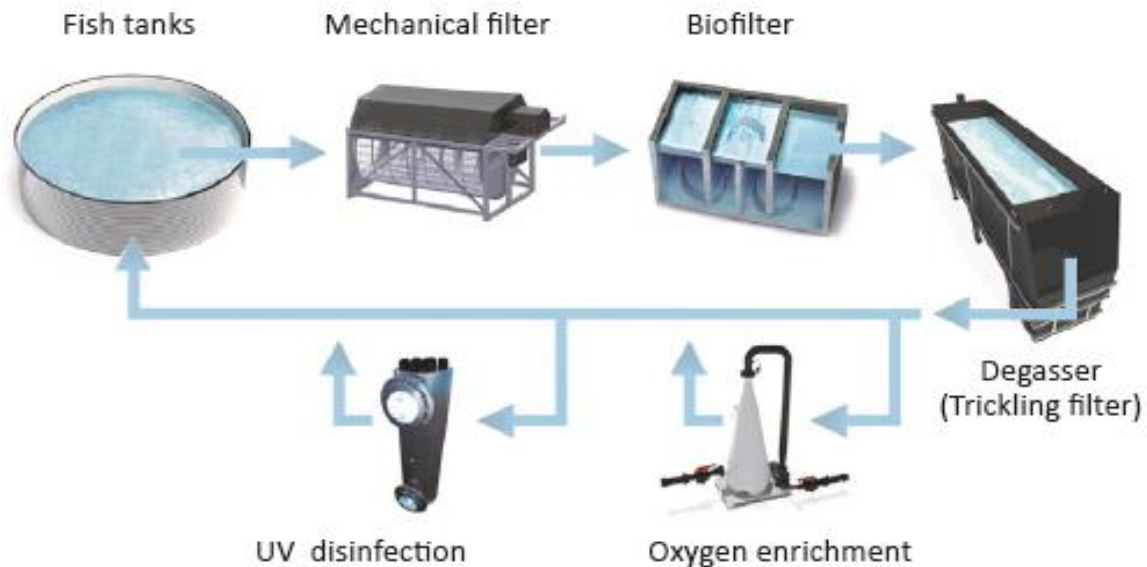
Figure 2. Principle drawing of a recirculation system (from Bregnballe, 2015).
