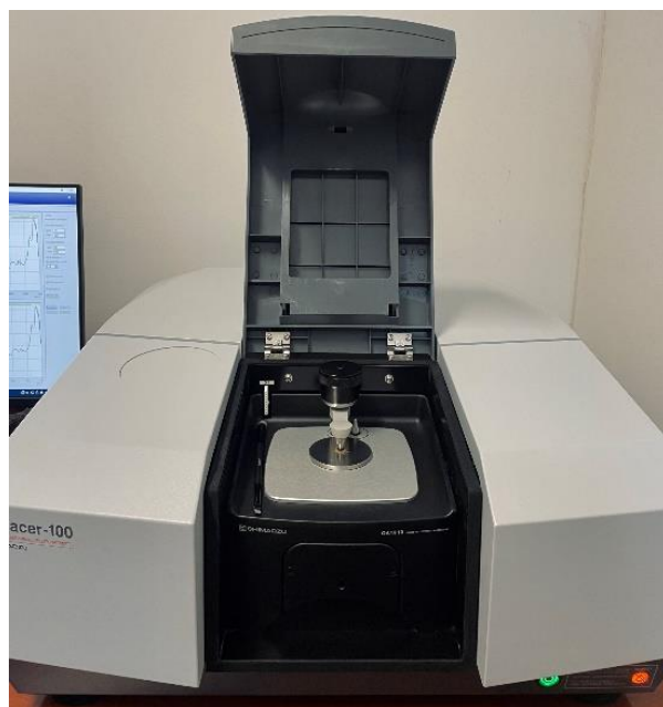
Figure 8. The FTIR-ATR spectrometer setup with the Shimadzu IRTracer 100 Spectrometer and single-reflection diamond ATR accessory **.
