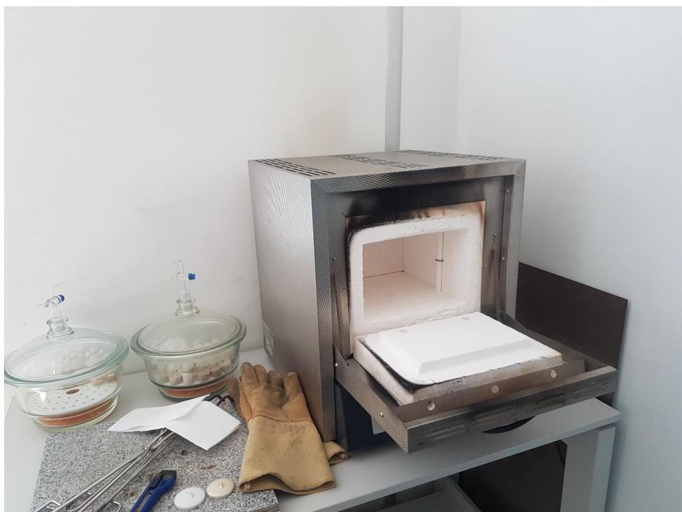
Slika 10. Mufolna peć marke Nabertherm Controller B170
