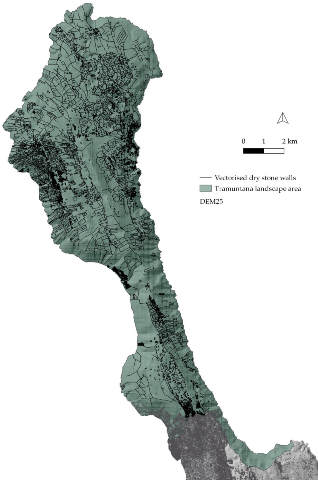
Figure 144. Vectorised dry stone walls of the Tramuntana landscape unit Area: 92.54 km 2 , Length: 1,284.09 km, Density: 13.88 km/km 2 (138.8 m/ha)
