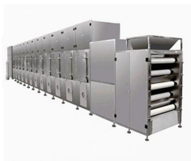
*Slika 16. Trakasta sušara (<https://sudaneseyha.net/conveyor-dryer-machine/ce-approved-screen-printing-conveyor-dryer-belt-machine-for-sale.html>)*
