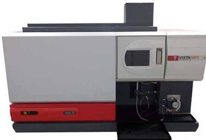
Slika 3.7.3.2.1. Uređaj ICP-OES Vista MPX (Varian)
