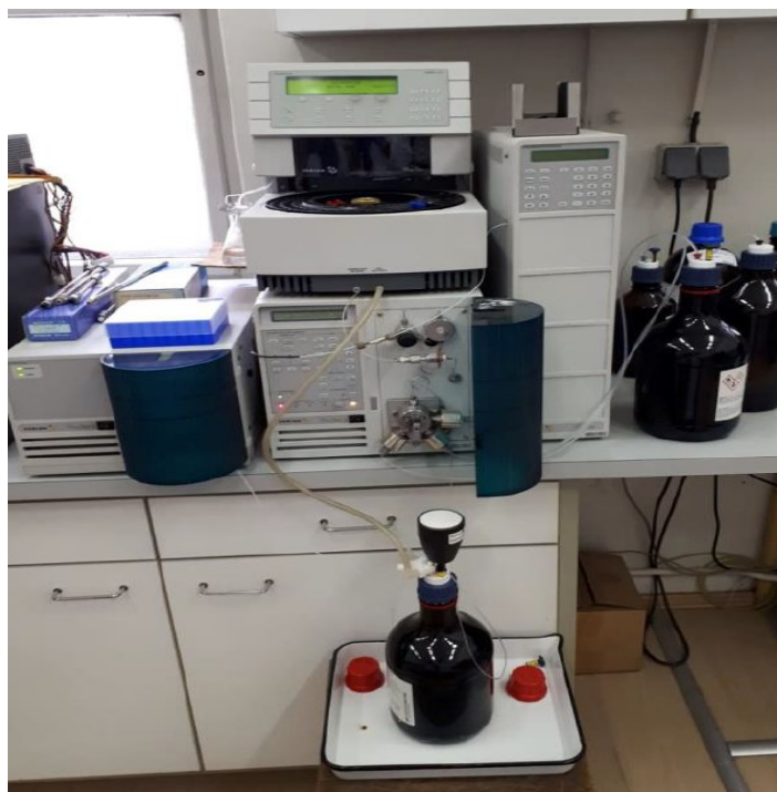
Figure 12. Varian ProStar 500 HPLC system used in quantification of extracted pyrethrins.
