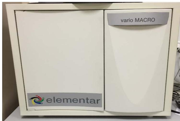
Slika 18. C,H,N,S analizator
